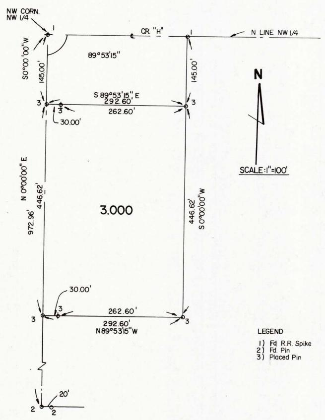
"I do hereby certify that I have surveyed the premises and prepared the attached plat and that the plat is correct."
